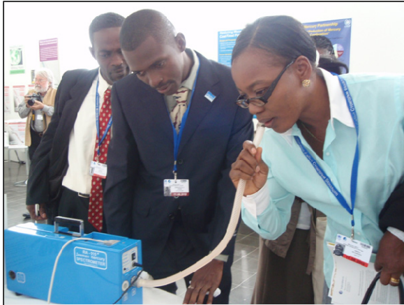
The Lumex machine being used during INC sessions as part of the 'Say ...aaaHg!' initiative to measure mercury levels coming mainly from dental amalgams.
